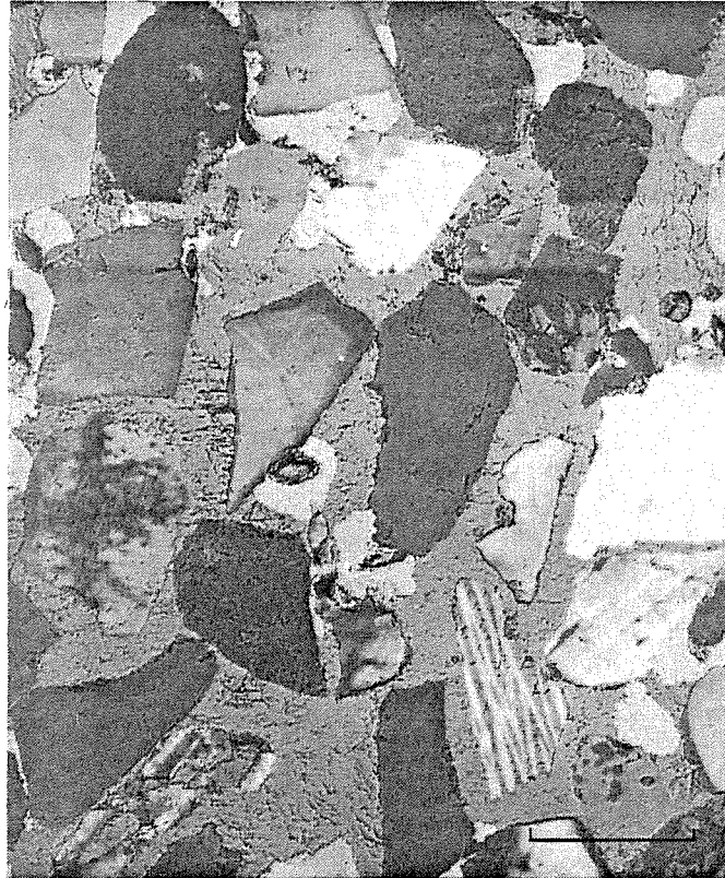
Figure 3.3.7 Combined cathodoluminescence and back scatter image showing siderite (white) occurring as inclusions in calcite (light grey). Clastic grains (various shades of white to dark grey) show syntaxial quartz and feldspar cement predating calcite cement. Sample 48.80 m. Bar is 0.1 mm.
