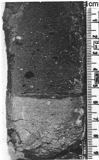
Figure 6.11 Sharp boundary between glacial sediments and Tertiary sedimentary rocks at site 7316/06-U-02.
