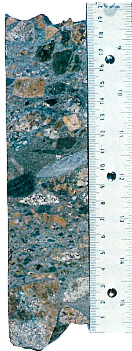
Fig. 6. 25/10, core 9, 3020 m. Polymict conglomerate of probably Rotliegendes age.
