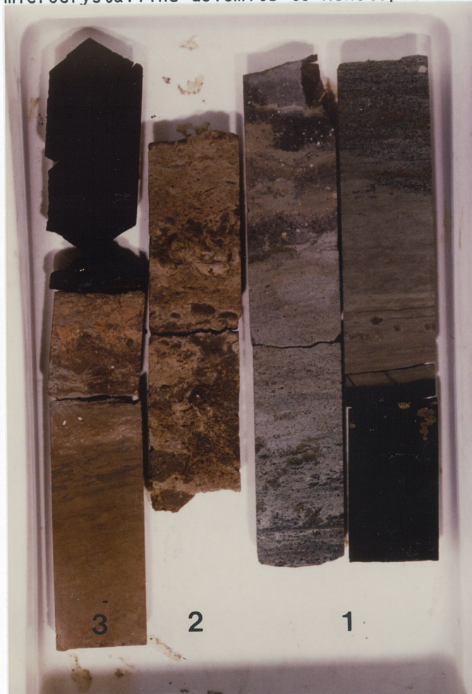
Fig. 4.3 Units A, B and C, and lithological boundaries in core D85-J. Part 1 shows the abrupt change from unit A to B. The lower part of unit B contains abundant clastic grains and glauconite. Part 2 shows the interval 30.37-30.66 m of wackestone-packstone with mouldic porosity as small black spots. Part 3 (29.73 to 30.20 m) shows the change from wackestones in B to black and dark grey silty claystone at the base of C.
