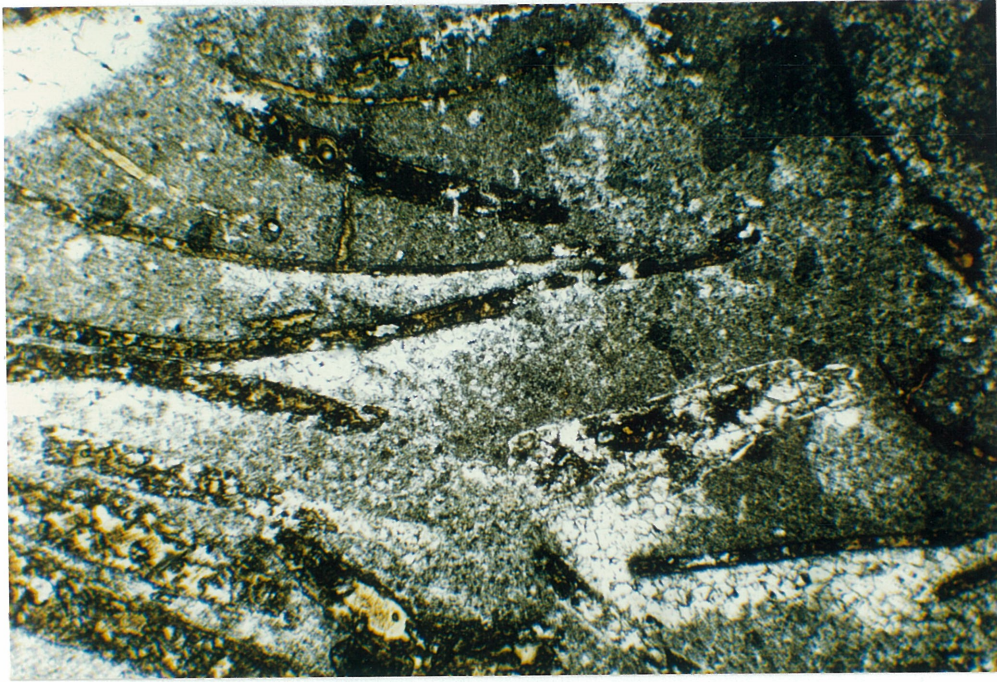
Fig. 4.5 A partially dolomitized packstone in plane polarized light. The brown and black coloured areas are partially dissolved Buchia fragments. The dark and fine-grained areas are dominantly microcrystalline calcite (micrite), the white areas are drusy calcite and dolomite cements. Dissolution of Buchia fragments took place later than precipitation of the calcite and dolomite cements. Sample 30.93 m.
