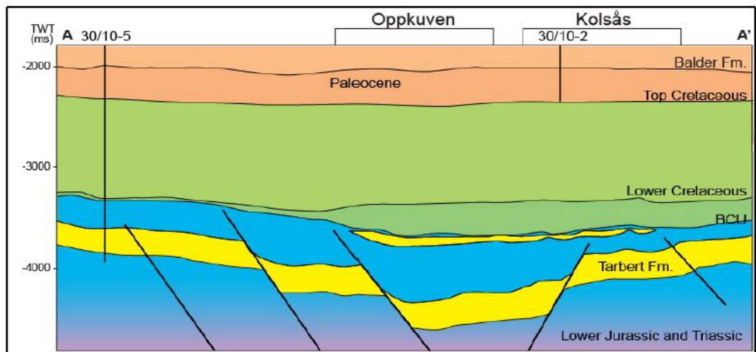
Fig. 1.2 Geoseismic section of the Kolsås S prospect. *Kolsås S, Oppkuven and Kikut prospects along line A-A'.*
