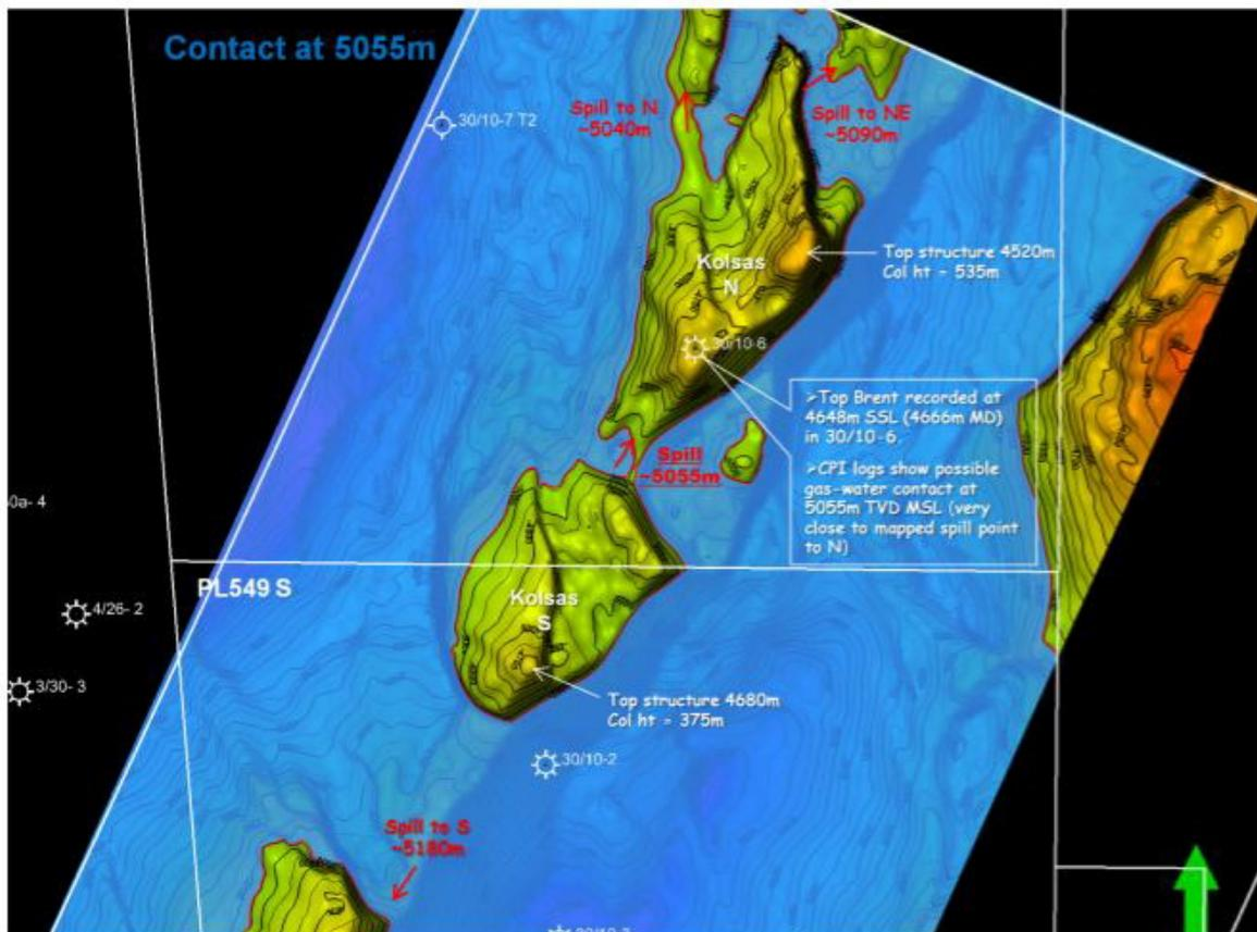
Fig. 1.3 Top Brent depth map. Top reservoir depth map with 375m column height and spill towards north.
