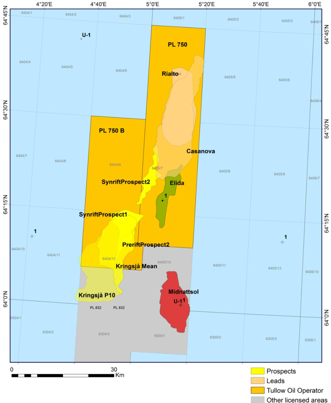
**Fig. 1.1 License prospect and leads.** *The Cretaceous Kringsjå prospect, Casanova Lead and Rialto Lead. The pre-Cretaceous Synrift prospect 1 & 2 and Prerift 1 Prospect.*
