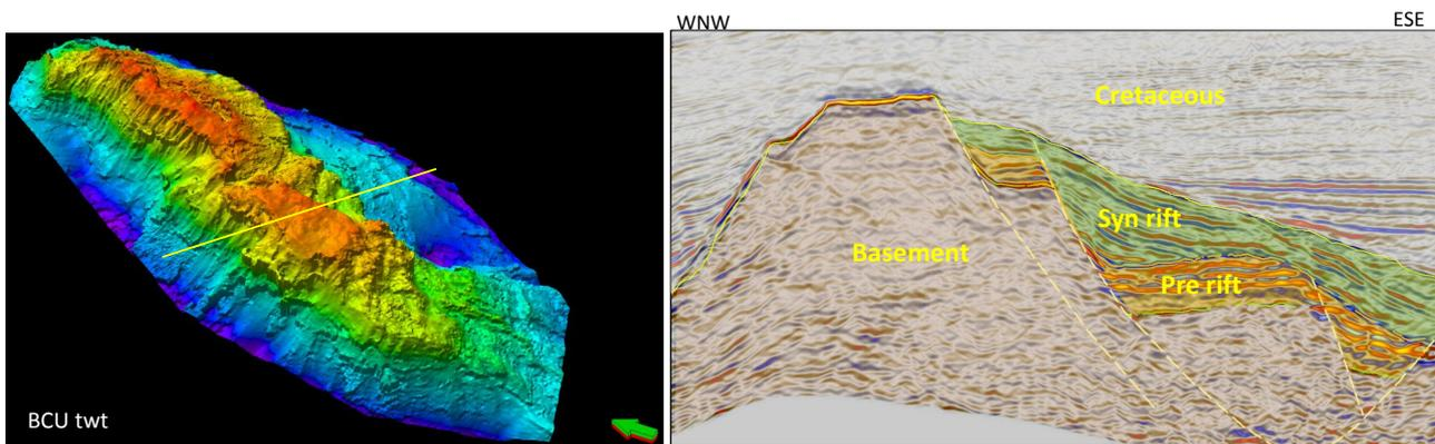
**Fig. 4.4** Seismic cross section across the Grip High. The cross section illustrates the separation of the pre-Cretaceous strata into a separate tectonostratigraphic units
