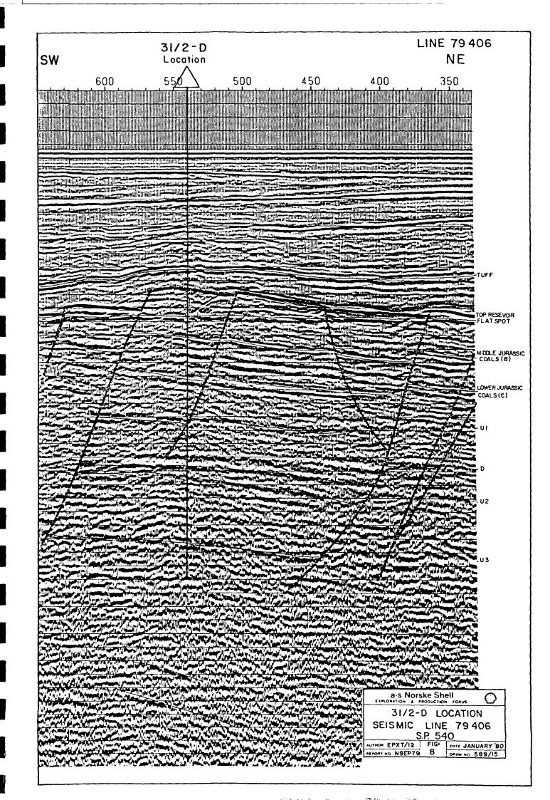
Depth conversion of this time map has not been attempted because of uncertainties about the reliability of velocity determinations beneath the Jurassic section in the presence of residual multiple energy. For depth estimations at the proposed location an interval velocity of 3500 msec has been used between the Top Triassic and the D reflection. Error estimates for the deeper part of the hole reflect the rapidly increasing uncertainty with depth.
