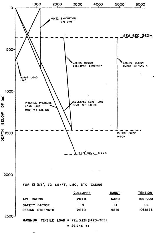
13 3/8", 72 LB/FT L80, BTC CASING IS THEREFORE SATISFACTORY IN BURST, COLLAPSE AND TENSION FOR THIS WELL.
