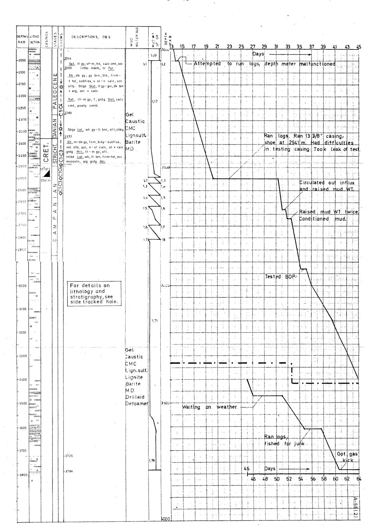
Fig A.2 (cont.) DRILLING PROGRESS, WELL 30/7-6
