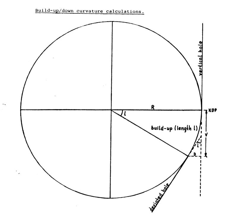
The dog-leg is defined as change in indination per drilled length (s degrees over a distance 1). The correlation between s, 1 and the radius R is then:  $R = \frac{180 \ 1}{\Pi \ s}$  and further we have:  $V = R \sin i$  (i is the deviated hole inclination)  $D = R - R \cos i$  $M = \Pi Ri/180$
