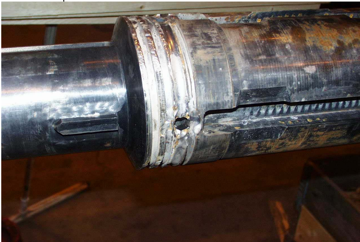
Washout in all 4 port on 9 5/8" Floating Junk Bonnet BA.
