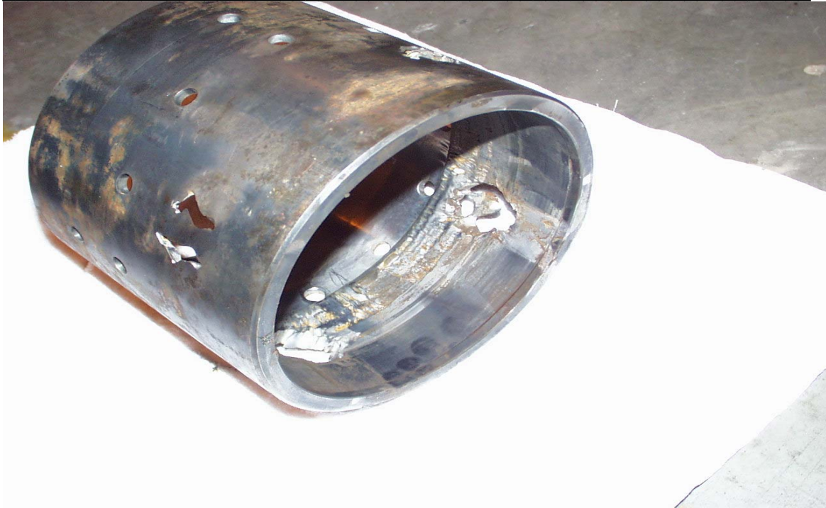
Washout in equalizer sleeve.
