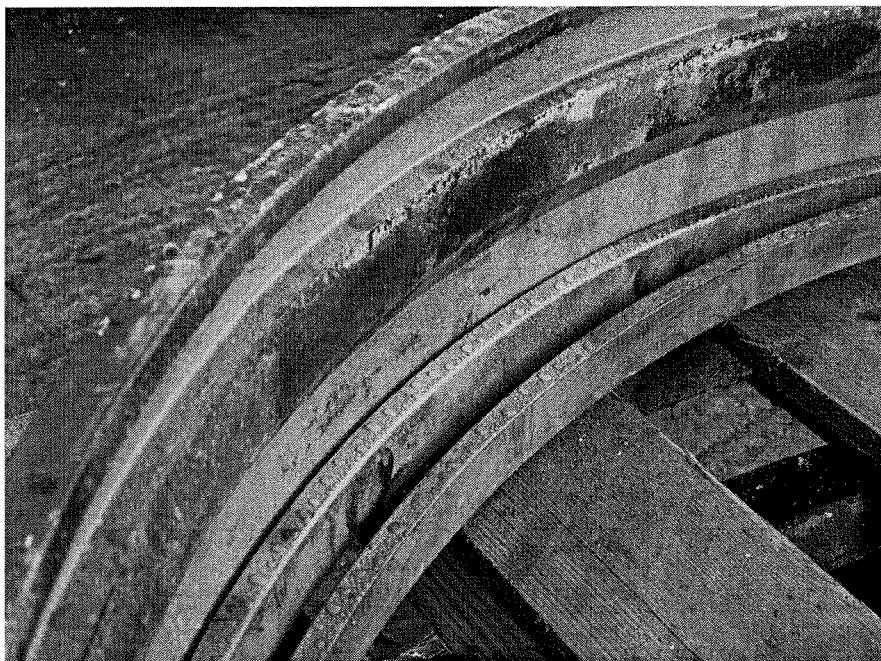
Typical damage to drive sleeve internal profile
