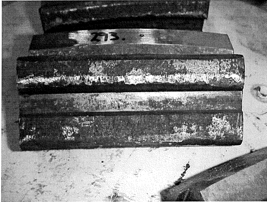
Typical damage to face of dog segments
