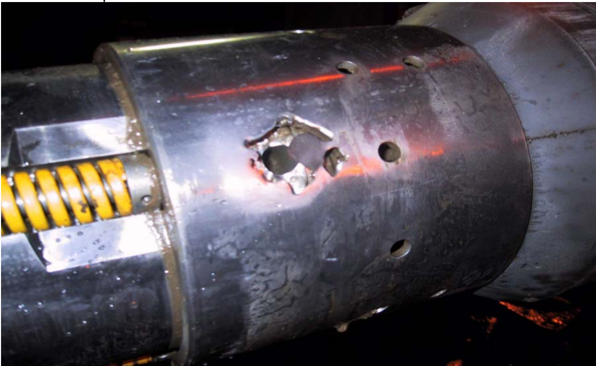
9 5/8" Floating Junk Bonnet BA. Picture taken on West Alpha when tool on surface.
