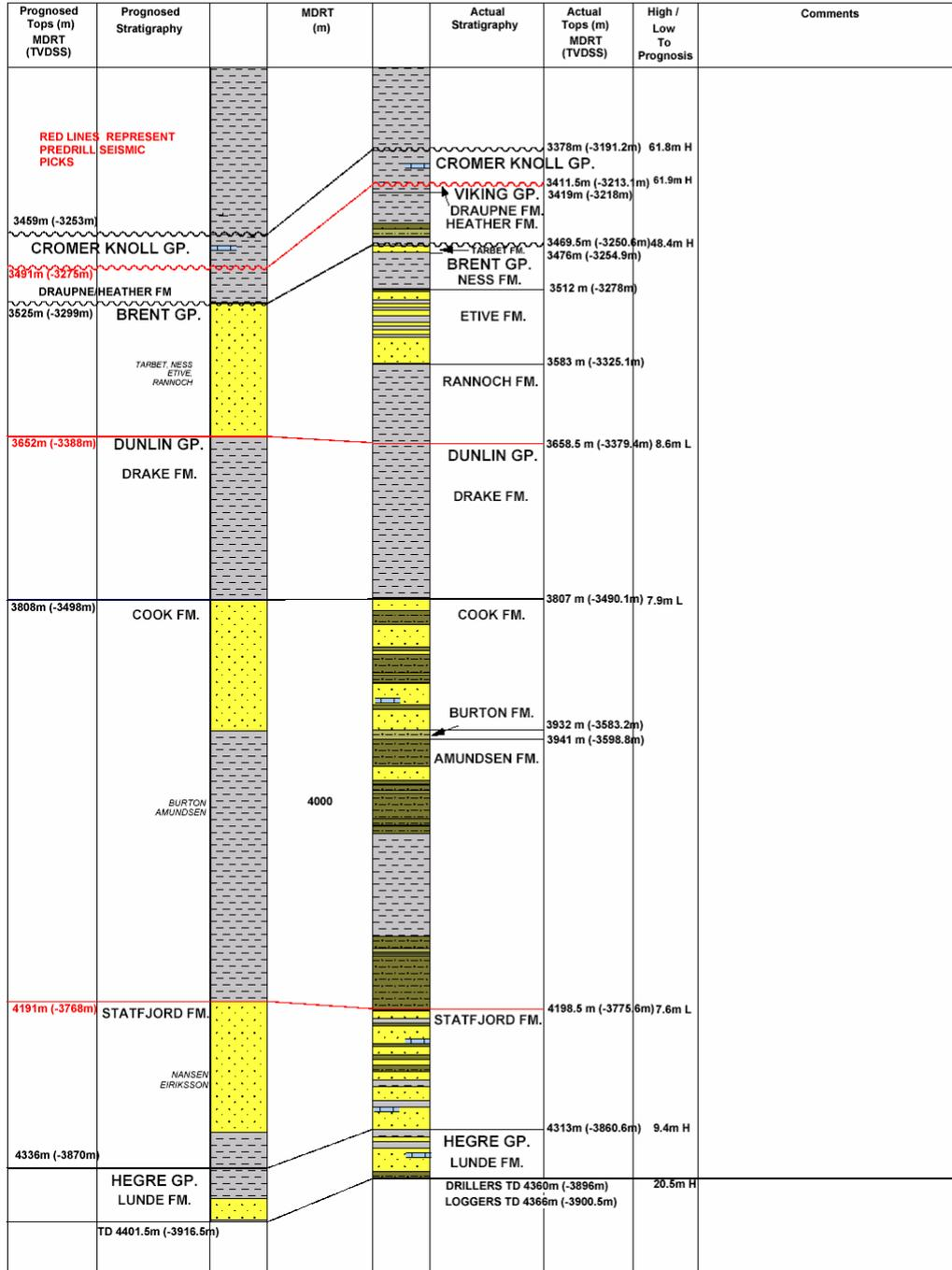
Figure 5 Geological Column Prognosed vs Actual – Detail of Reservoir Section
