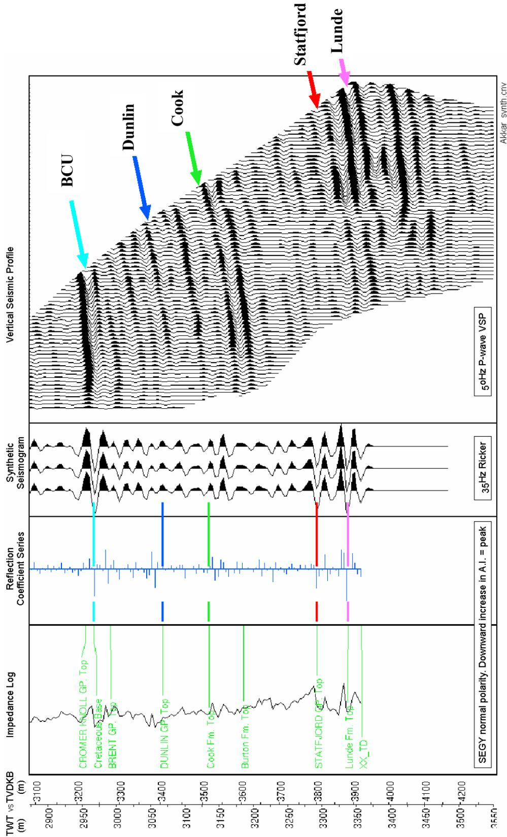
Figure 3. Composite well tie display showing impedance log, reflection coefficient series and resulting synthetic seismogram together with VSP for comparison. Horizon ties on VSP panel are indicated by respective coloured arrows.
