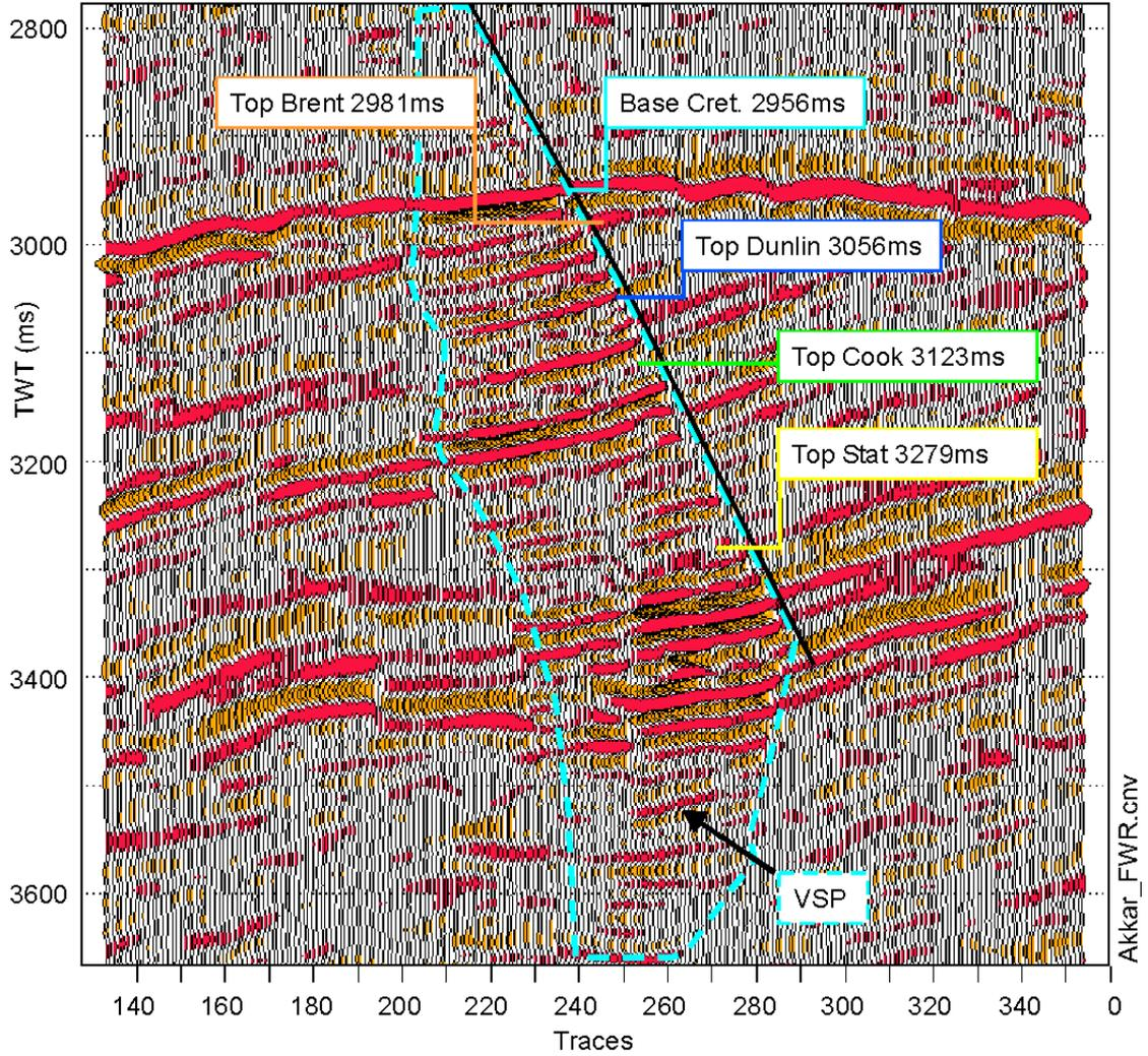
Figure 2. Zero phase VSP spliced into surface 3D seismic with -25ms shift applied. Surface seismic is an arbitrary line along the well path taken from the cn01m02 survey. SEGY normal polarity i.e. downward increase in acoustic impedance = peak (red).
