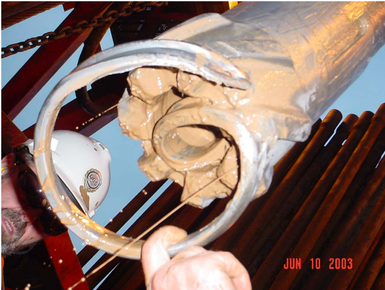
Core head w/junk from the 16" casing hanger assembly
