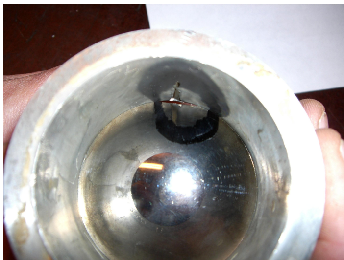
Figure 8-1: LPR-N ball valve after test
