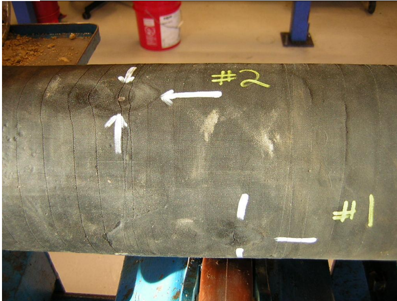
Figure 6-2: Packer elements after cased hole MDT
