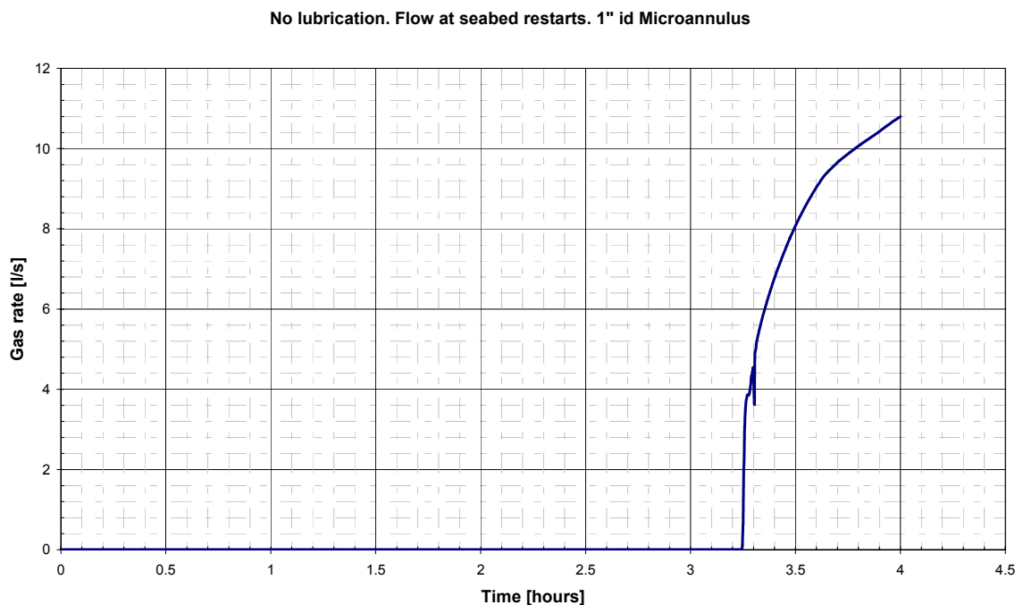
Figure 5.4: Gas restarts at seabed 3 hours after well has U-Tubed and stabilized (approximately 50 meters of air in top of riser).
