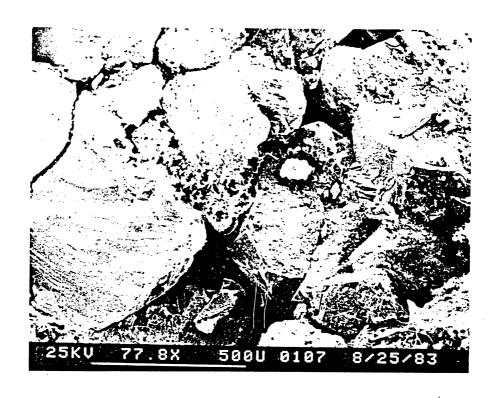
**Figure B4.** Overview. Note large grains, large open pores. Dissolved feldspar in upper center part of photograph. From 3717.35 meters, permeability given above.
