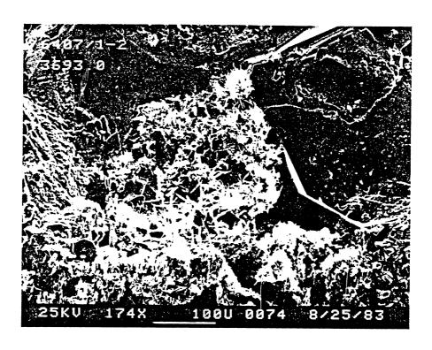
Figure B16. Fibrous illite growing on quartz overgrowths. From 3693.0 meters.
