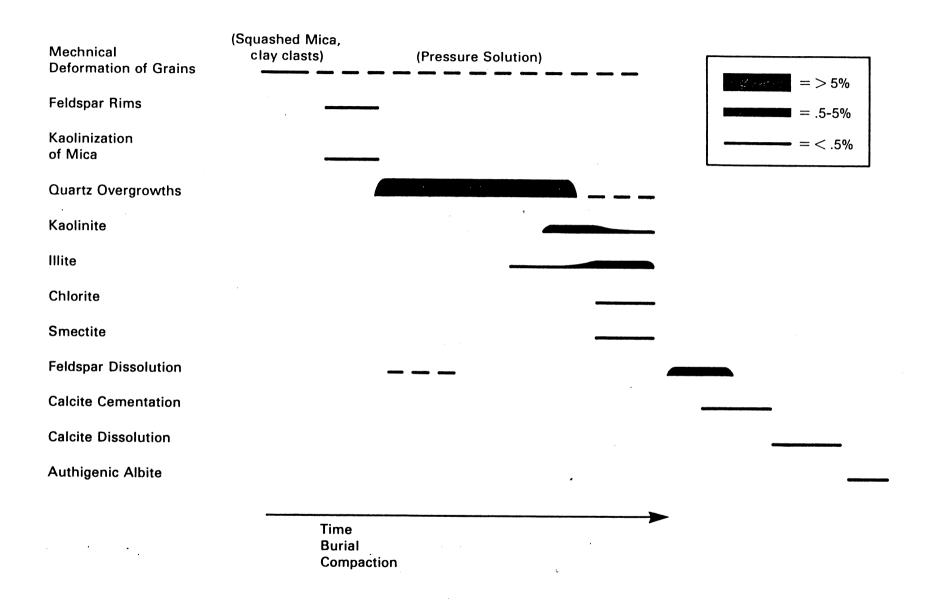
Figure 3. Sequence of diagenetic events. Volume contribution to porosity is indicated by the height of the bar.
