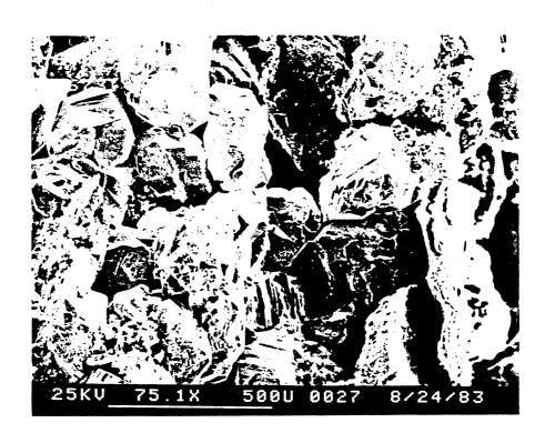
**Figure B8.** Abundant quartz overgrowths. Dissolved feldspar just below center. Squashed mica in lower right. From 3673.4 meters.
