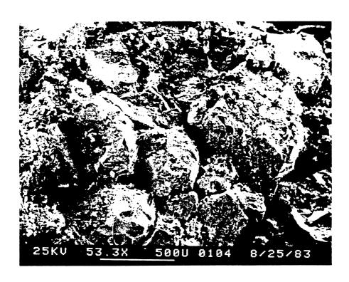
**Figure B3.** Overview. Note large grain size and relative lack of quartz overgrowths. Larger, more open pore throats are present. Permeability is 168 millidarcies. From 3717.35 meters.
