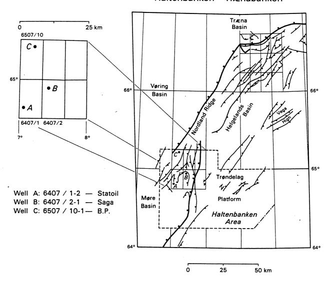
**Figure 1.** Major structures in the Haltenbanken area, offshore Norway, showing location of wells discussed in this report. Downthrown side of faults is indicated by tick marks. Displacement rarely exceeds 500 meters. Modified after Aesheim and Larsen (in press).
