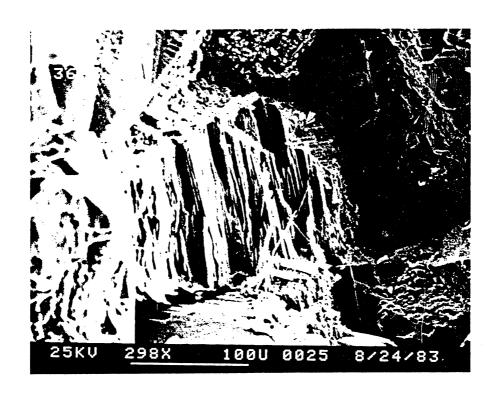
**Figure 5.** SEM photograph of dissolved K-feldspar grain from 3673.4 meters. Quartz overgrowths on right and illite at bottom.
