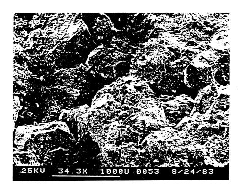
Figure B2. Overview. Quartz overgrowths and authigenic clay are present. Permeability of this sample is 119 millidarcies. From 3699.35 meters.
