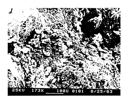
**Figure 6.** Pore-plugging kaolinite from 3717.35 meters.
