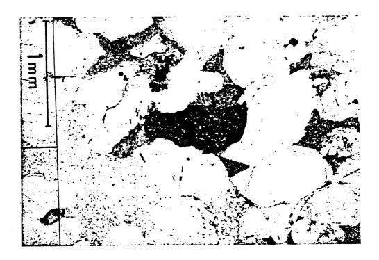
**Figure 4.** Photomicrograph of sample from 3717.35 meters. Quartz overgrowths are abundant. Squashed grain in center is volcanic rock fragment. Note abundant kaolinite filling pores. Dissolved feldspars (2) just above rock fragment and right center.
