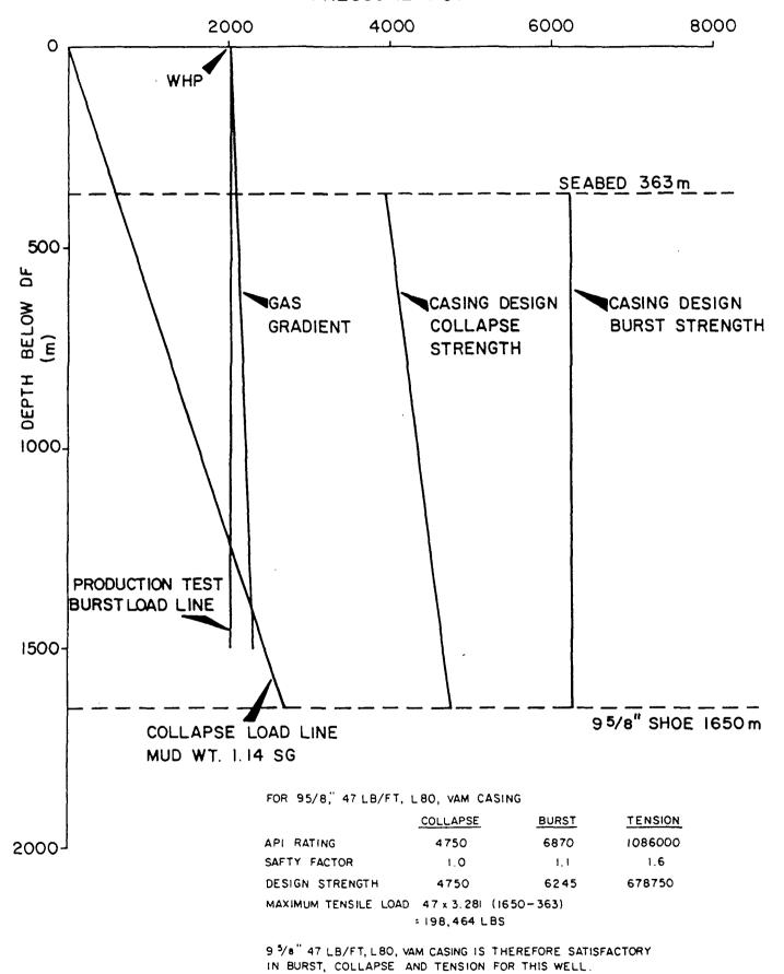
THE DESIGN SHOWS THAT THE CASING CAN WITHSTAND A PRODUCTION TEST ON THE MAIN GAS RESERVOIR.
