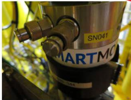
Figure 3-3 Location of the 3 4Subsea Motion sensor installed on BOP for Zulu
