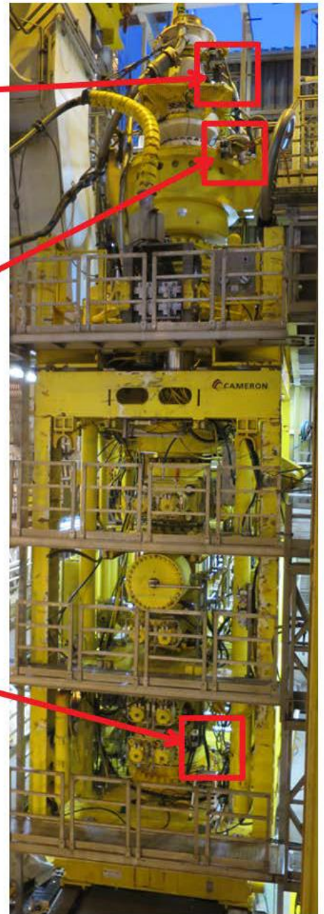
Figure 3-3 Location of the 3 4Subsea Motion sensor installed on BOP for Zulu
